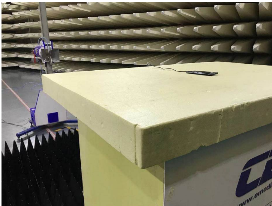
Spurious Radiated Emissions Test setup
