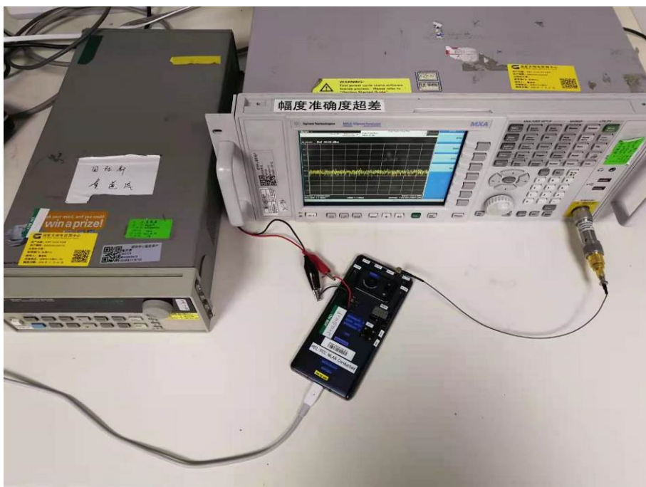
RF Conducted Test setup (BT/WIFI)
