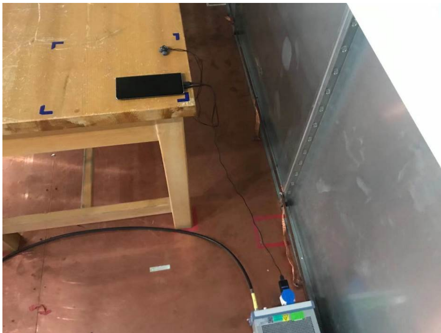
Conducted Emissions Test Setup (with charger)
