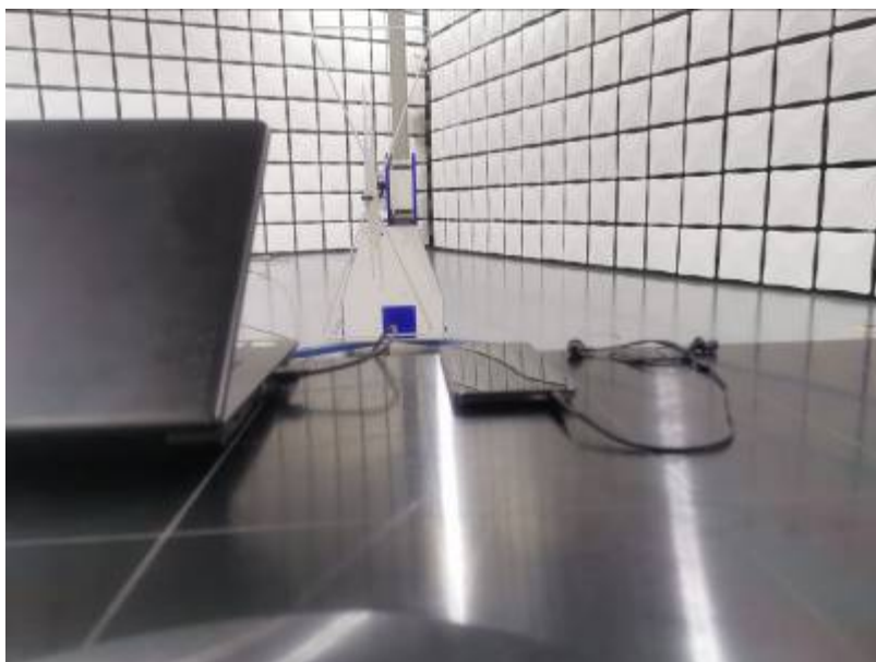
Radiated Emissions Test Setup (30-1000MHz)
