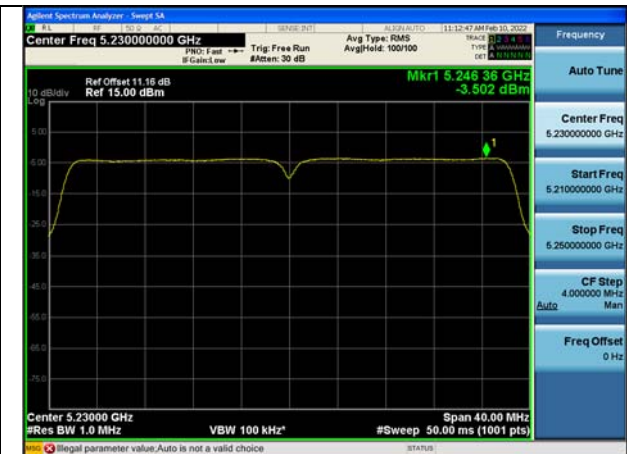
Test Mode:802.11n HT40 5230MHz Chain0
