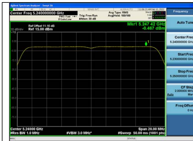
Test Mode:802.11n HT20 5240MHz Chain0
