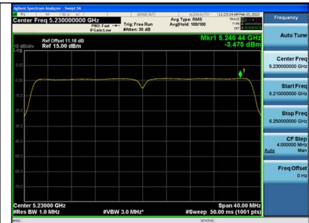
Test Mode:802.11ac VHT40 5230MHz Chain0
