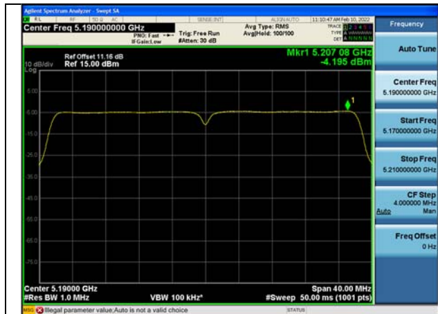
Test Mode:802.11n HT40 5190MHz Chain0
