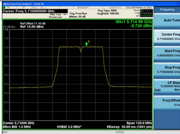
Test Mode:802.11ac VHT40 5710MHz Chain0 NII2C
