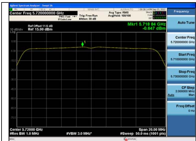
Test Mode:802.11n HT20 5720MHz Chain0
