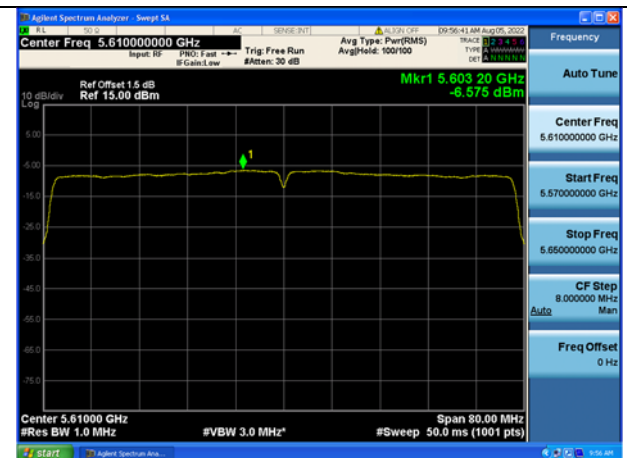
Test Mode:802.11ac VHT80 5610MHz Chain0
