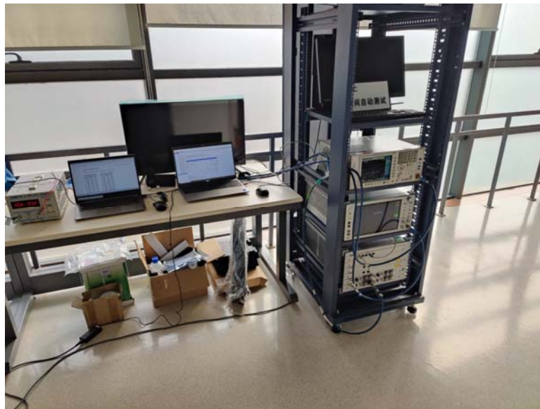
RF Conducted Test setup (LTE/NR)
