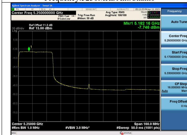
Mode:802.11ax HE160 Tone:484T Frequency:5250MHz Ant:Chain0
