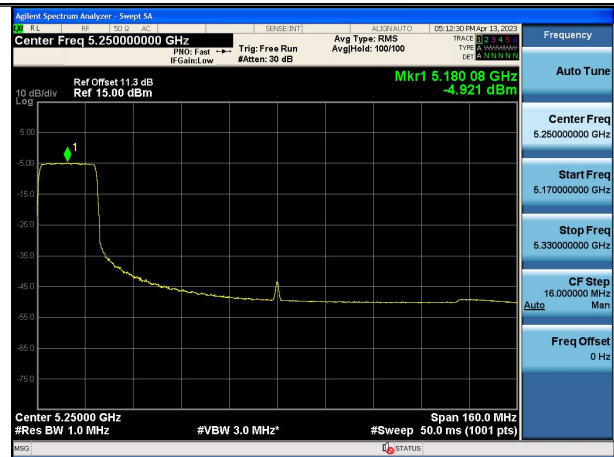
Mode:802.11ax HE160 Tone:242T Frequency:5250MHz Ant:Chain1
