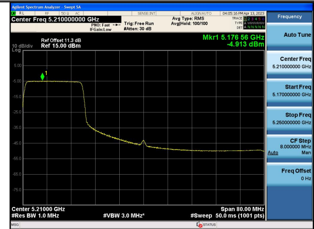
Mode:802.11ax HE80 Tone:242T Frequency:5210MHz Ant:Chain1
