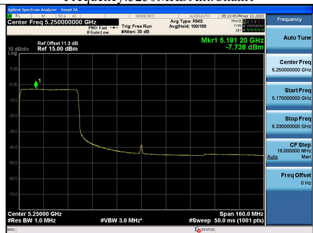
Mode:802.11ax HE160 Tone:484T Frequency:5250MHz Ant:Chain1
