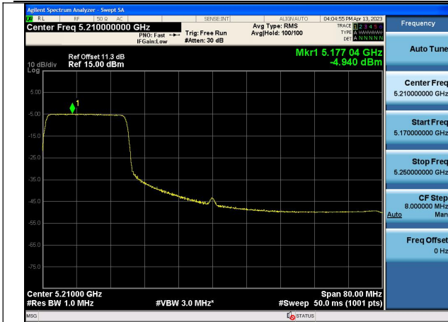
Mode:802.11ax HE80 Tone:242T Frequency:5210MHz Ant:Chain0
