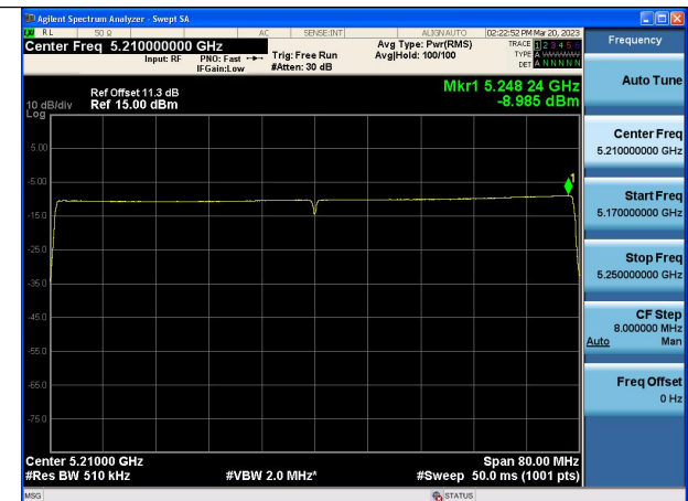
Mode:802.11ax HE80 Tone:996T Frequency:5210MHz Ant:Chain1
