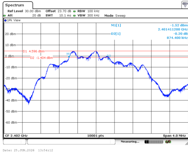
6 dB Bandwidth Plot on Channel 39
