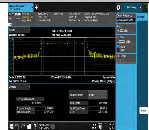
Band41-20MHz-QPSK-39750-100RB#0-PASS
