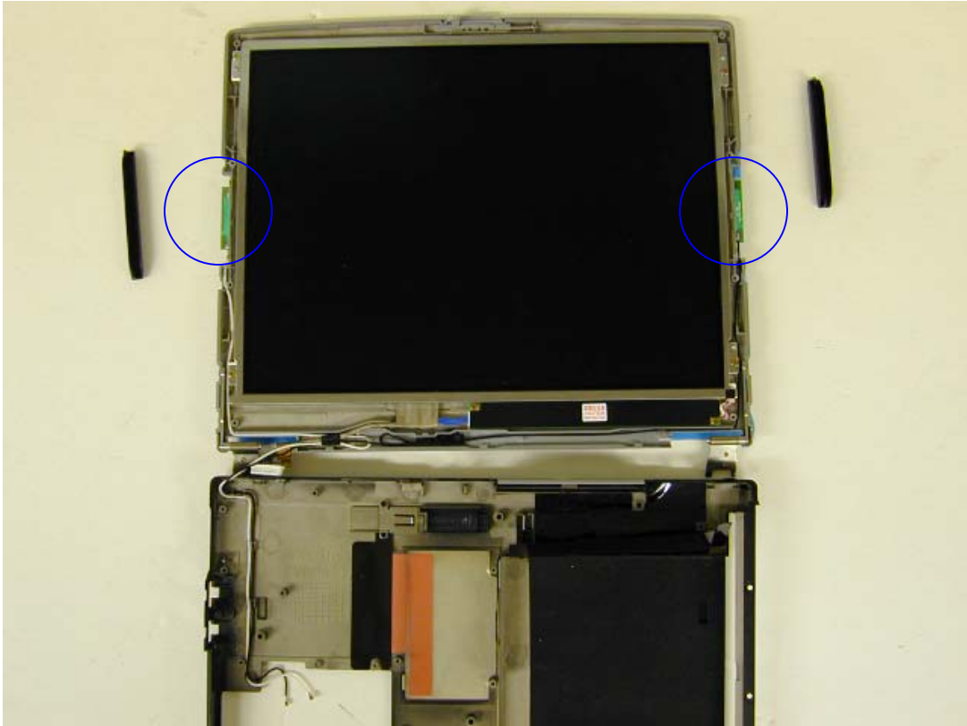
Location of Antennas
