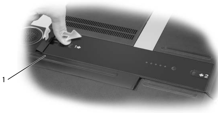
1 battery access door
