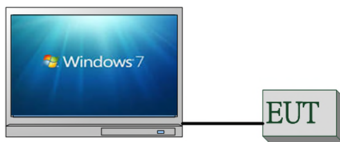
Fig. 2-1 Conducted (Antenna Port) & Radiated Emission & Conduction Configuration
