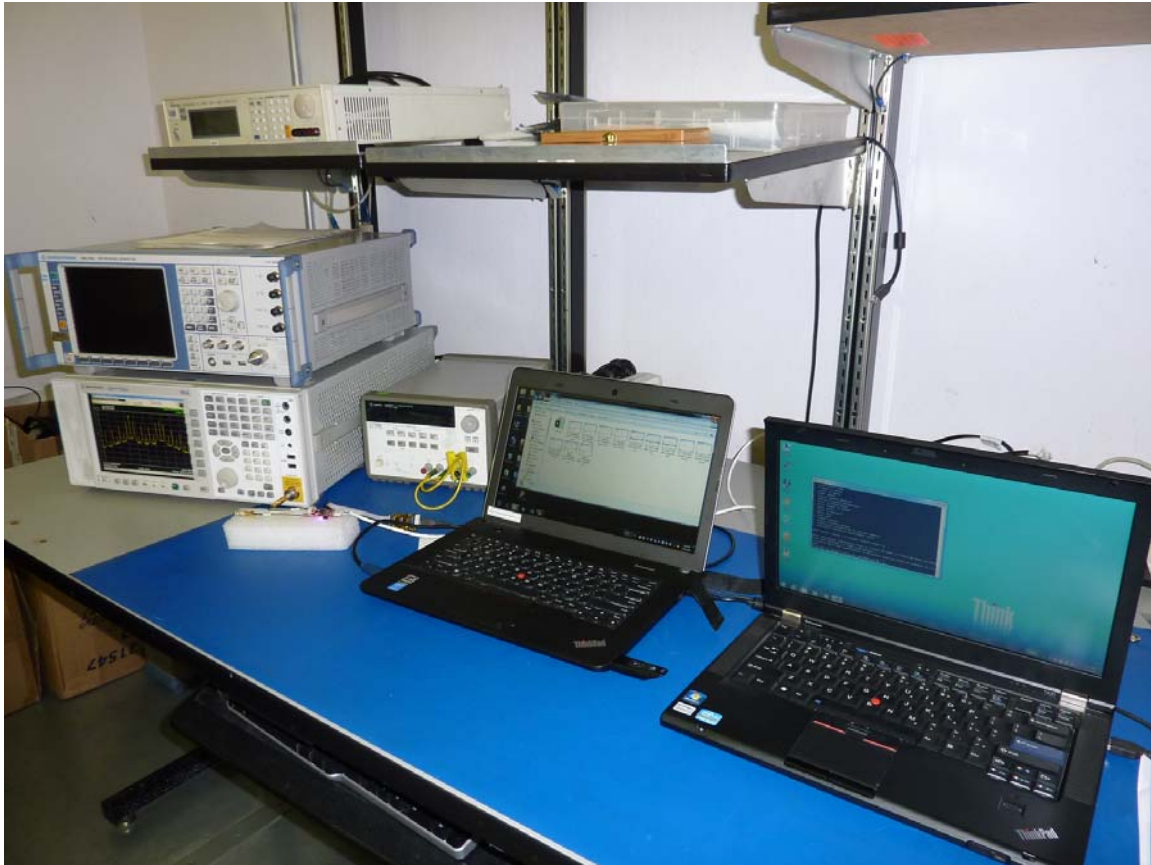
Figure 7: Conducted RF Test Setup
