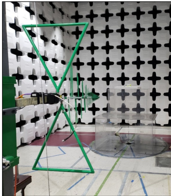
Photograph 2: Radiated Spurious Emissions Requirements, 30MHz-1GHz
