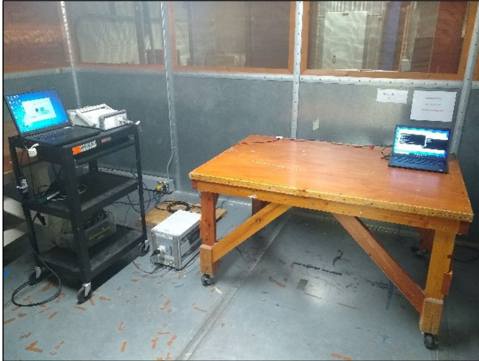
Photograph 3. Conducted Emissions Limits, Test Setup
