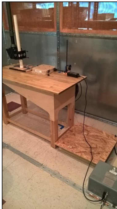
Photograph 16. Conducted Emissions, 5 Omni, Test Setup
