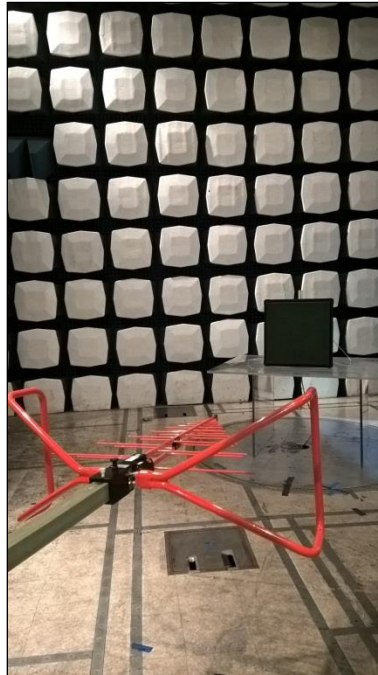
Photograph 3. Undesirable Emissions, 2' Panel below 1 GHz, Test Setup
