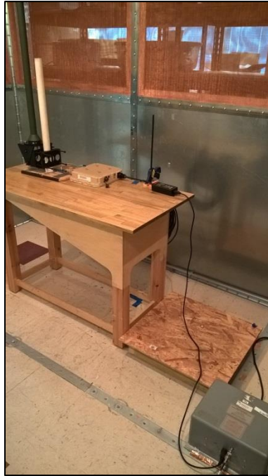
Photograph 17. Conducted Emissions, Omni 8, Test Setup
