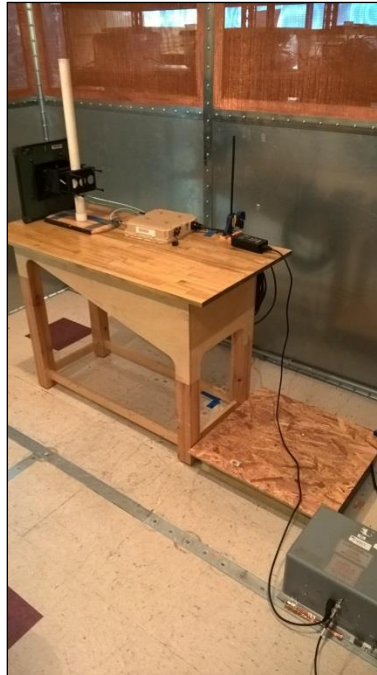
Photograph 13. Conducted Emissions, 1' Panel. Test Setup
