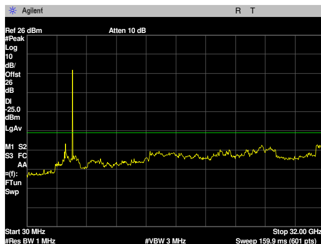
Plot 225. Conducted Spurious Emissions, 10MHz, 4945MHz, Port 2
