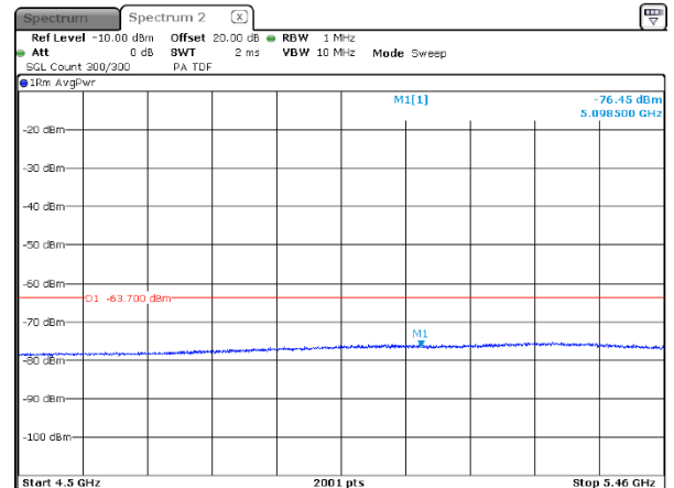
Plot 7.8.6 Conducted spurious emission measurements in the range 5.46 – 5.725 GHz
