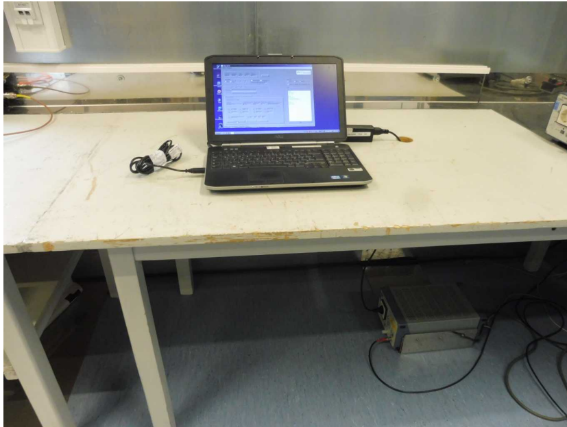
Photo 9: AC conducted emission test setup
