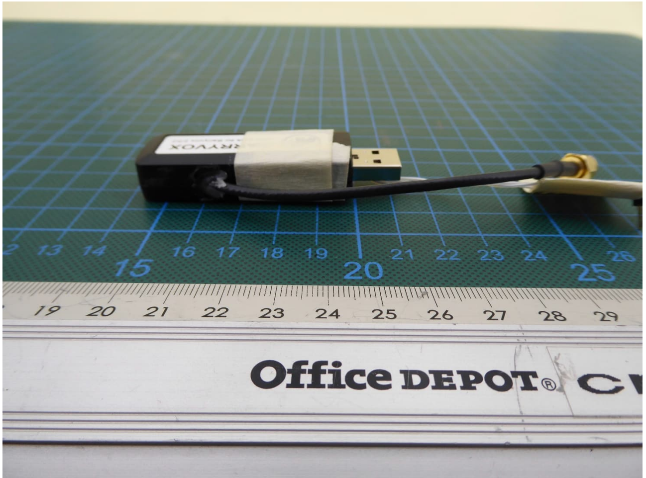
Modified EUT used for testing (conducted) – side view
