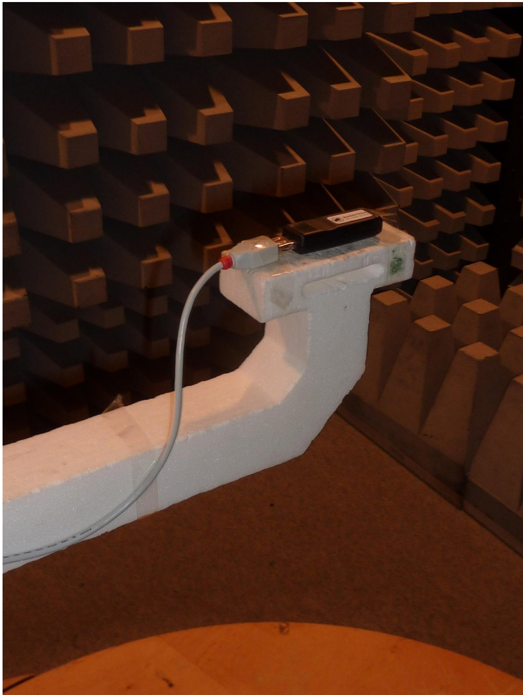
180803_1.JPG: W-LINK STICK, test setup fully anechoic chamber
