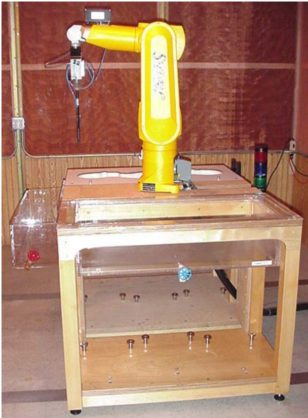
DASY4 SAR Measurement System with validation phantom
