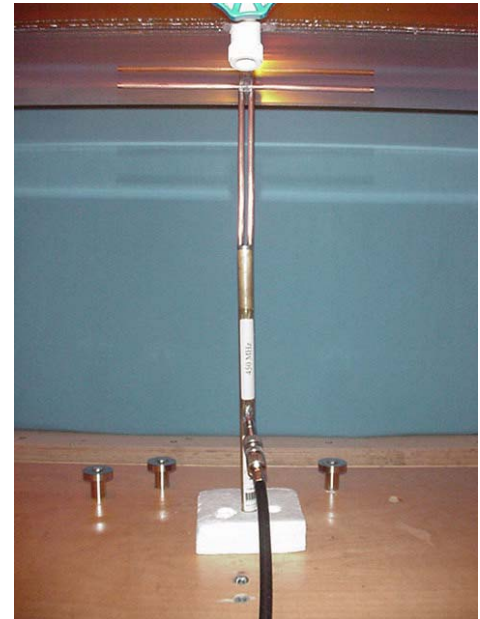
450MHz Dipole Setup
