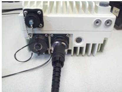
Figure 3-17 FullAXS cable, inner connector body in place
