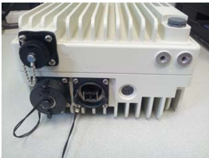
Figure 3-15 CPRI-S SFP port, exposed
