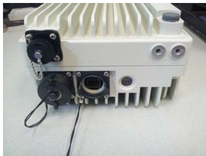
Figure 3-13 CPRI-S SFP cage, uncovered
