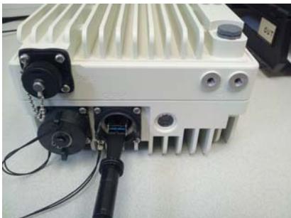
Figure 3-16 CPRI-S SFP port, LC connected
