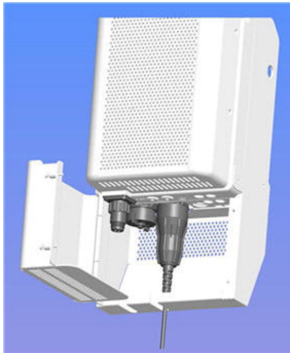
Figure 3-25 Security cover front attachment
