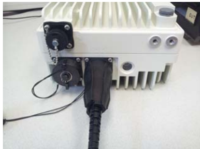
Figure 3-18 FullAXS cable, connected, and watertight
