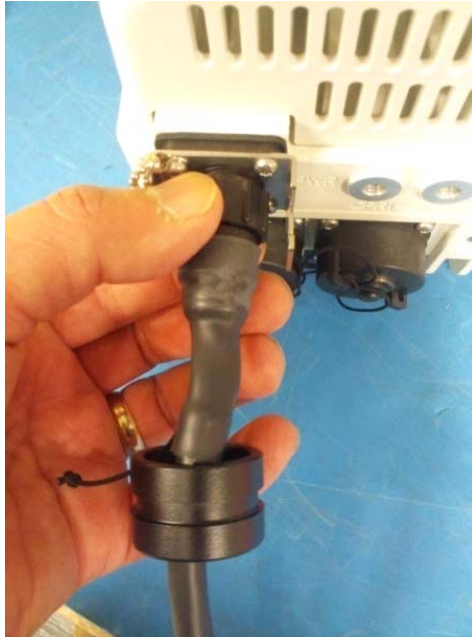
Figure 3-22 Power connector in the connector boot
