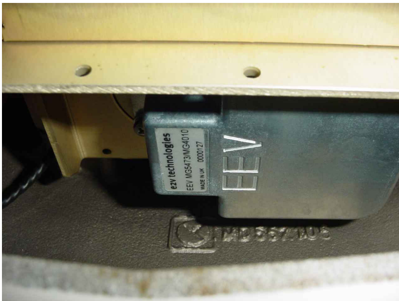
EUT, internal view, magnetron, labeling
