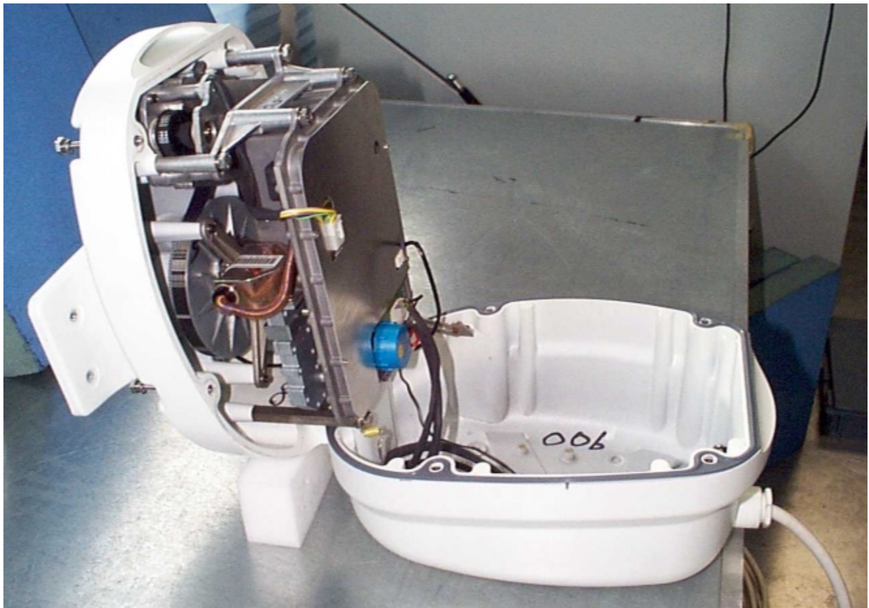
10kW, 48" Open Array Scanner Unit 10kW Pedestal – Internal view
