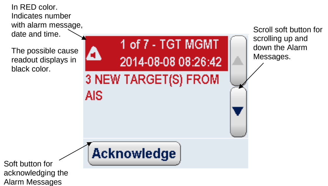
Figure 2-37 Display for alarm messages
