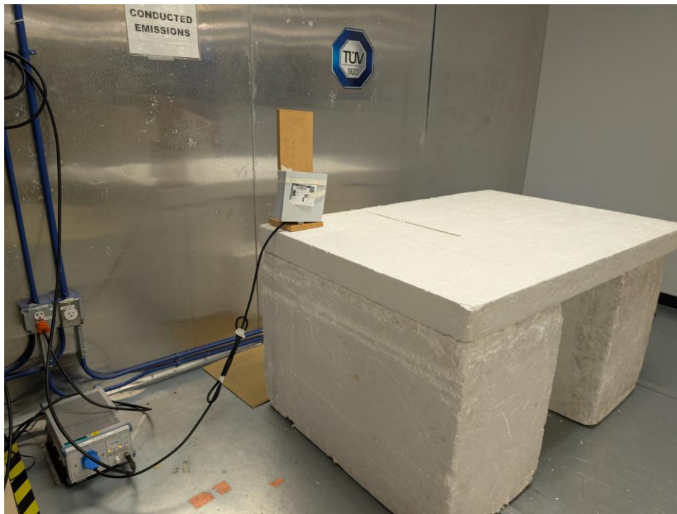
Figure:13 – Test Set up – AC Power Line Conducted Emissions
