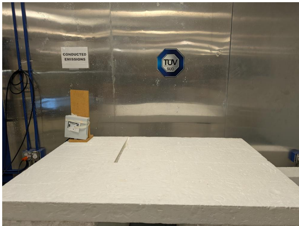
Figure:12 – Test Set up – AC Power Line Conducted Emissions
