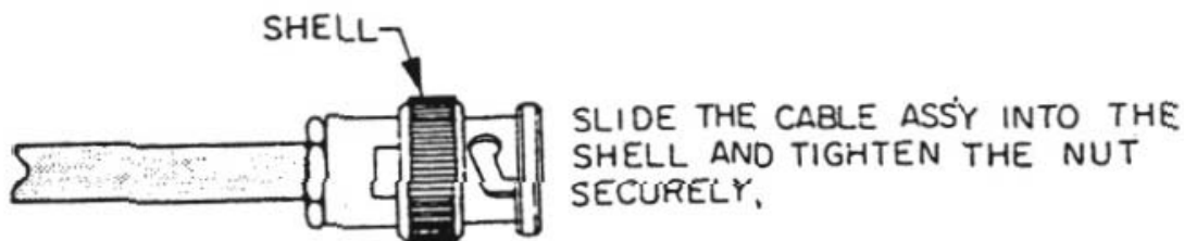
BNC Connector Assembly Procedure Figure 2017
