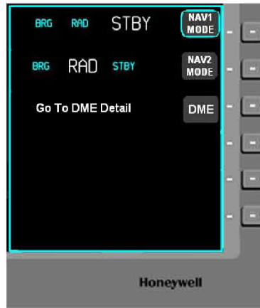
FIGURE 3-7 VHF NAV DETAIL WINDOW
