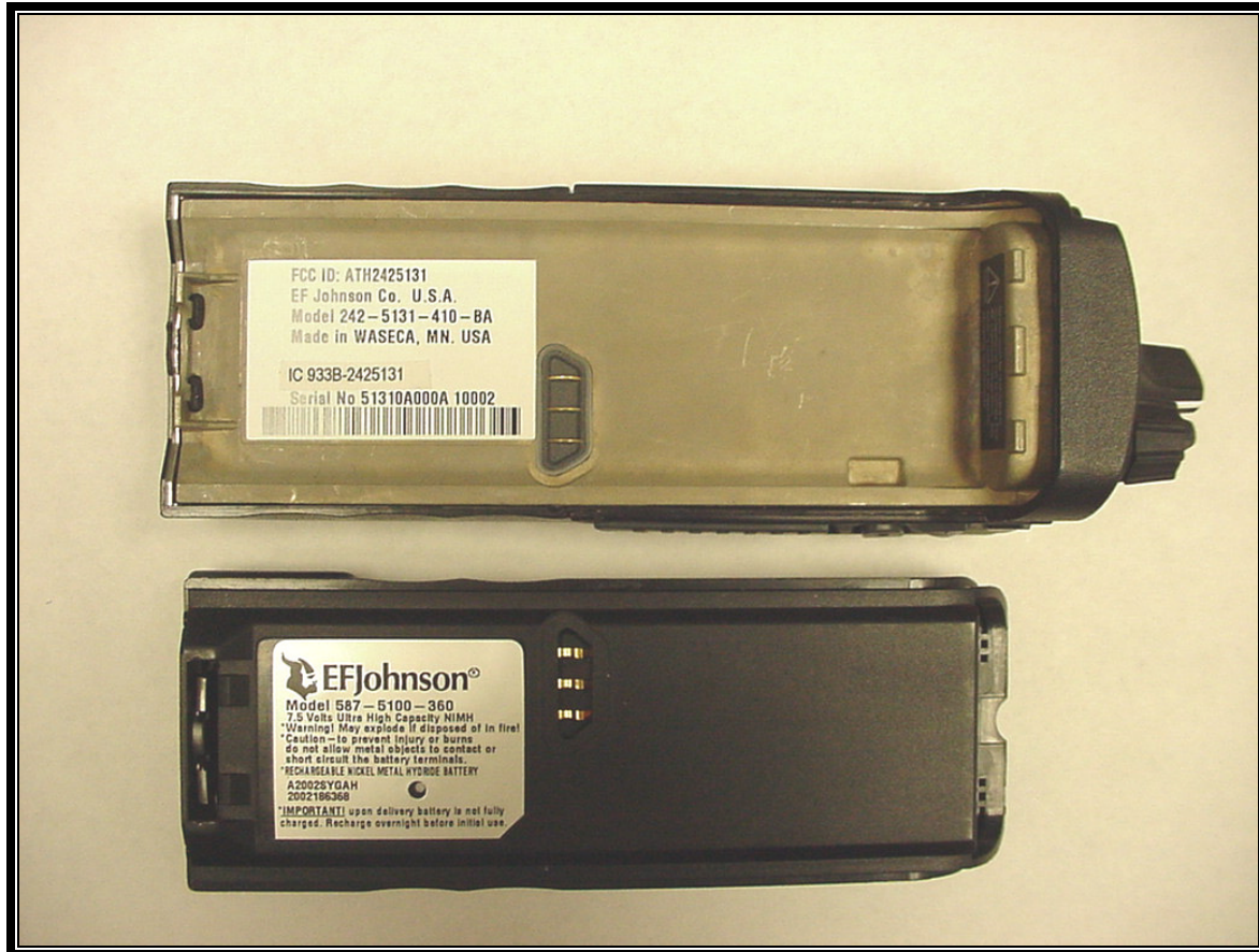
PHOTOGRAPH 12: BATTERY REMOVED FROM RADIO
