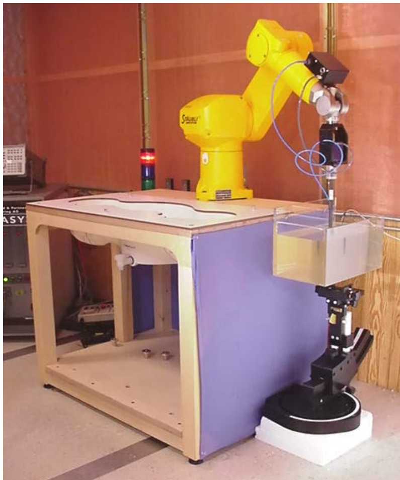
DASY3 SAR Measurement System with Planar Phantom
