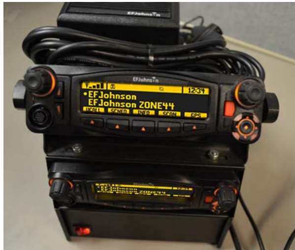
Figure 1.3 Viking Mobile Radio mounted in Base Station
