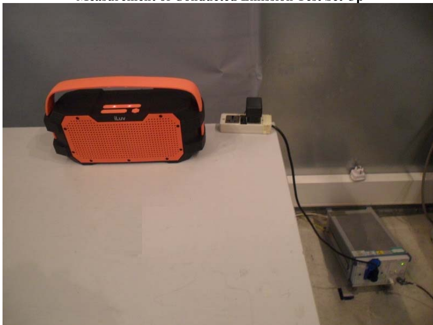
Measurement of Conducted Emission Test Set Up
