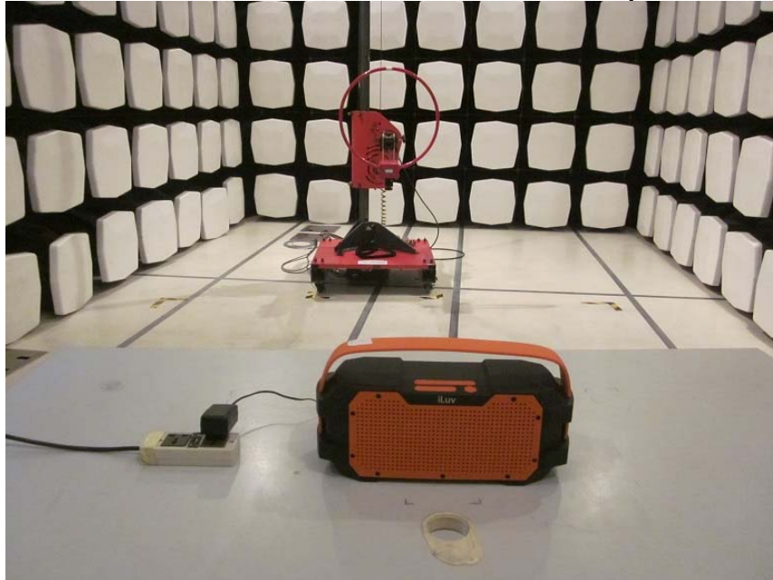
Measurement of Radiated Emission Test Set Up
