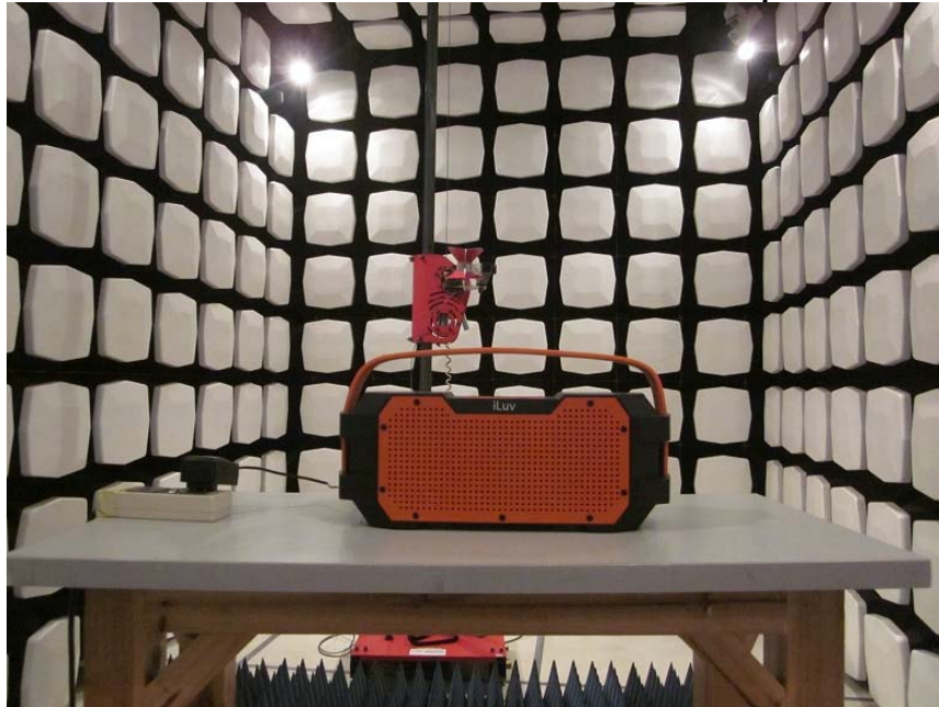
Measurement of Radiated Emission Test Set Up
