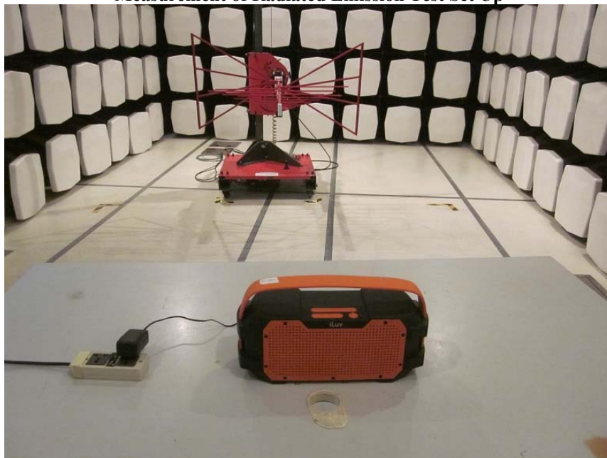
Measurement of Radiated Emission Test Set Up
