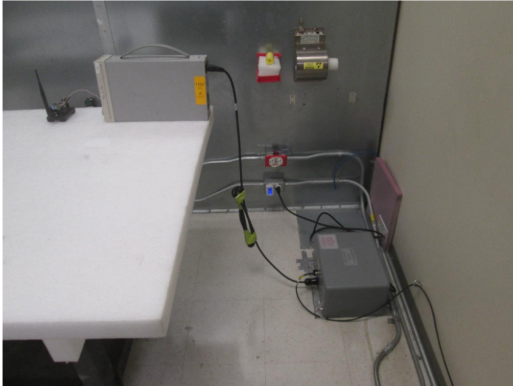
Power Line Conducted Emissions
