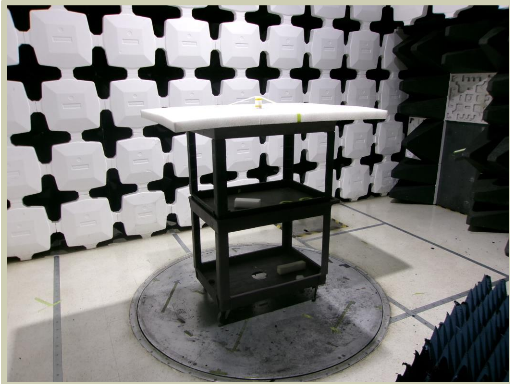
Set up above 1GHz
