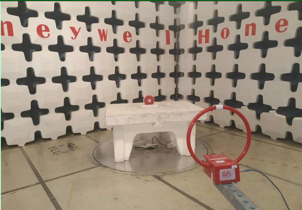
Radiated Emission Setup – 9 KHz to 30 MHz [ Parallel ]
