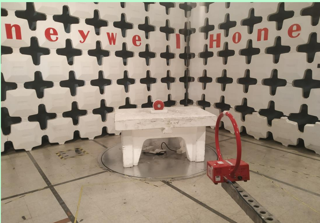
Radiated Emission Setup – 9 KHz to 30 MHz [ Perpendicular ]
