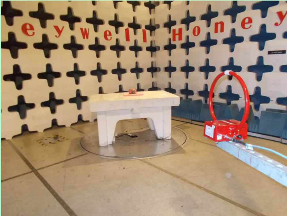
Radiated Emission Setup – 9 KHz to 30 MHz [Perpendicular]
