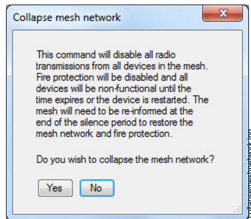
Figure 2.22 Collapse Mesh Network Option
