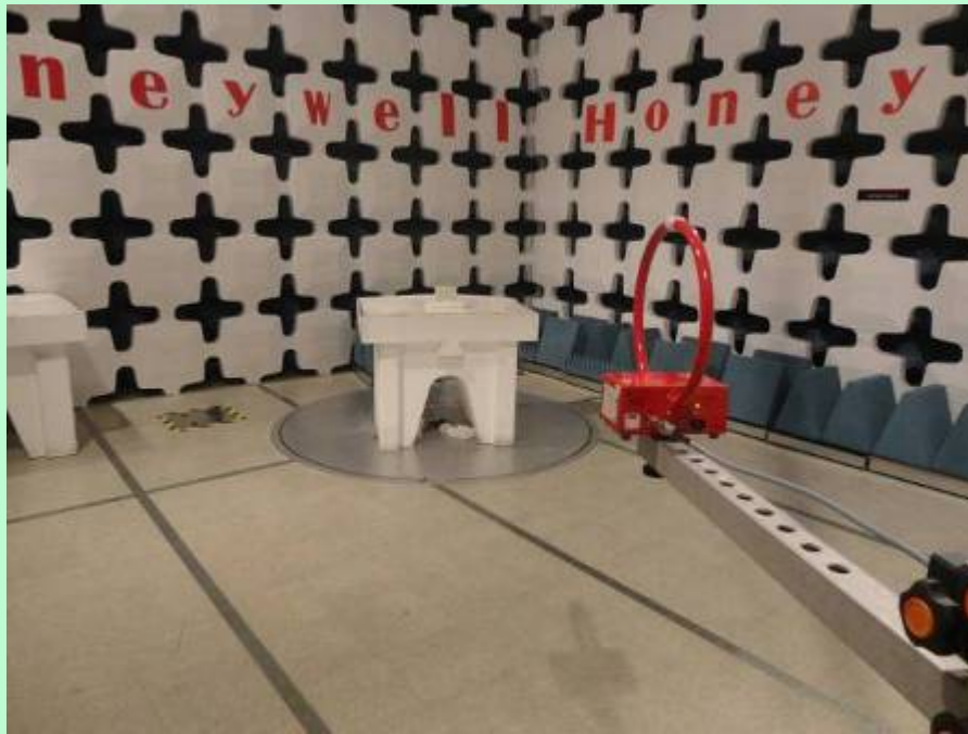
Radiated Emission Setup – 9KHz to 30MHz [Perpendicular]
