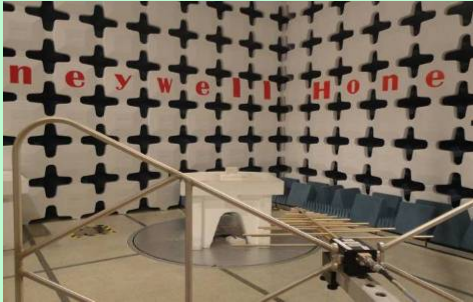
Radiated Emission Setup – 30MHz to 1GHz [ Horizontal Polarization ]
