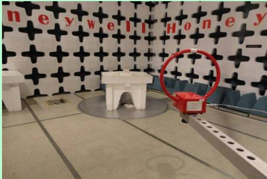
Radiated Emission Setup –9KHz to 30MHz [Parallel]
