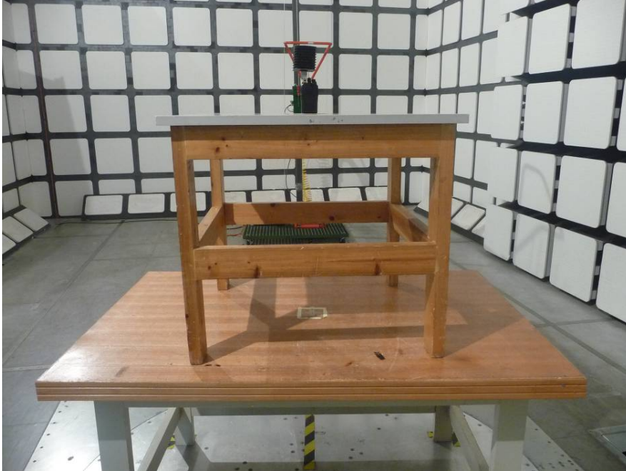
Transmitting Radiated Emissions (Below 1 GHz)
