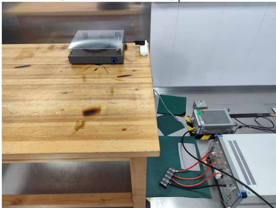
Conducted Emission at AC power line
