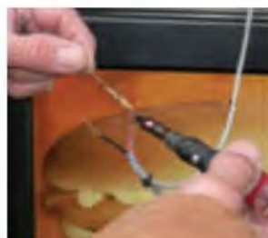
Fig.6 Solder all connections.
