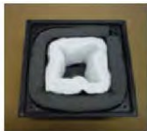
Fig.2 Install 3M foam and acoustic insulation.
