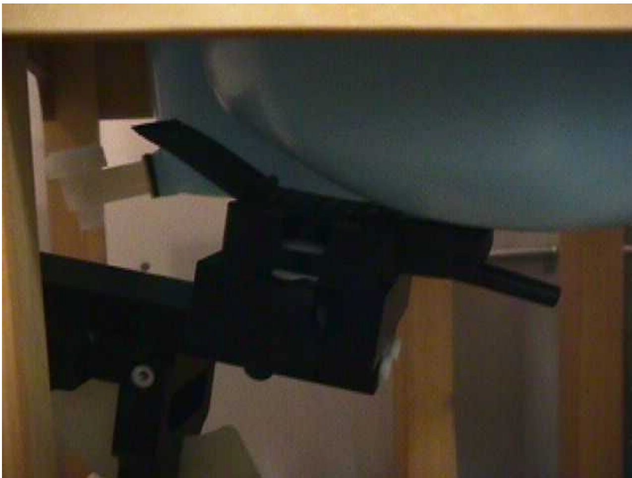
Fig. 7: KF 788 position under the left side of the DASY3 head phantom, top view.
