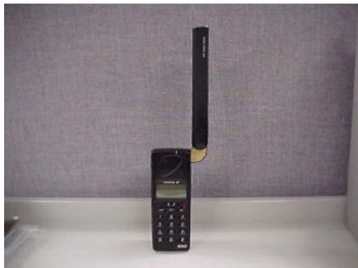
Front view of device for the four user positions of the antenna, (a) the stowed position, (b) the left-hand user position, (c) the 180° position, and (d) the right-hand user position.
