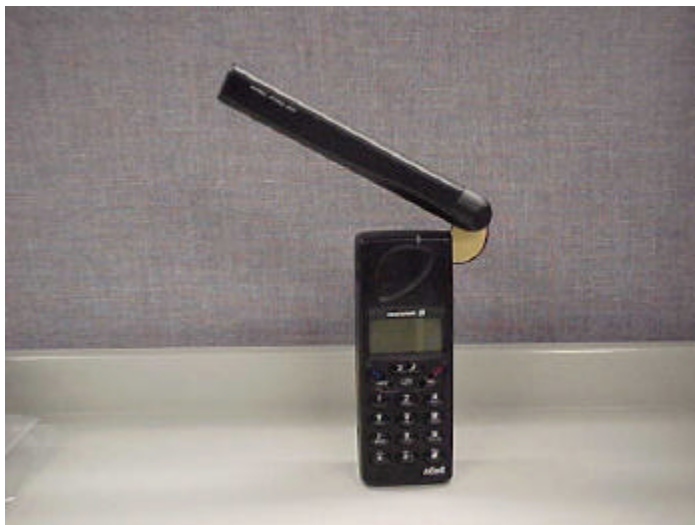
Front view of device for the four user positions of the antenna, (a) the stowed position, (b) the left-hand user position, (c) the 180° position, and (d) the right-hand user position.
