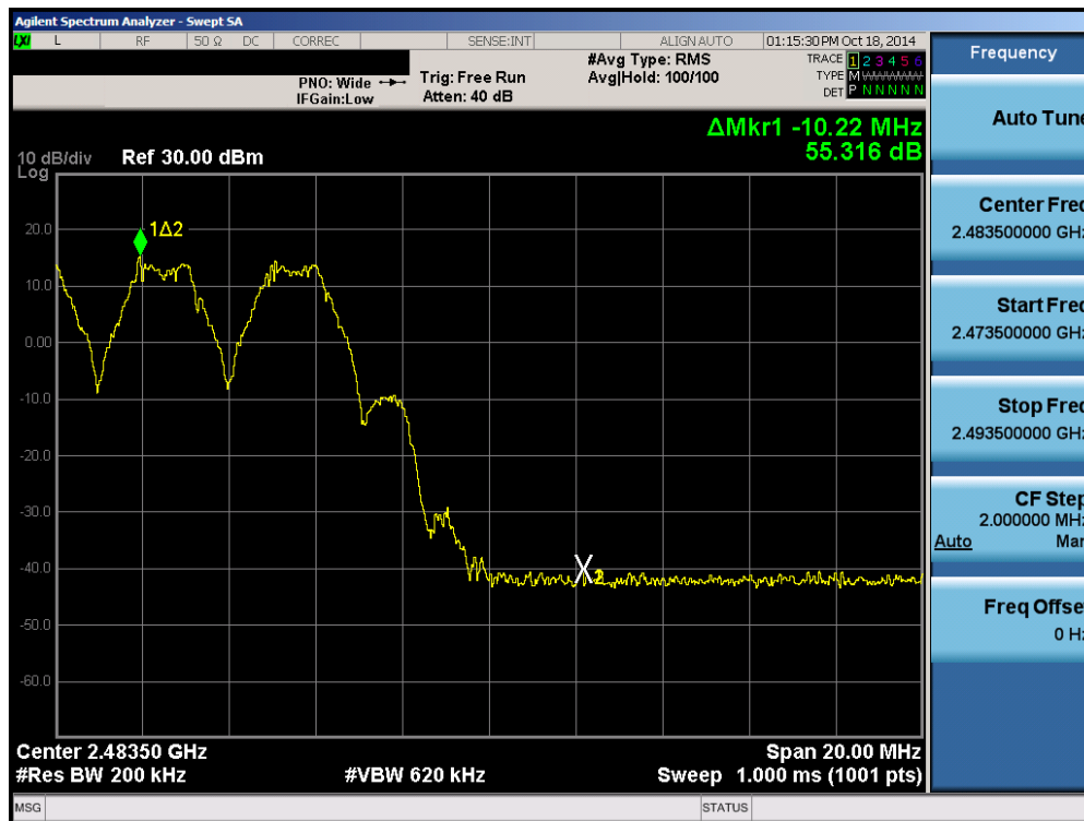
Plot 6-10. Band Edge Plot (Hopping Enabled)
