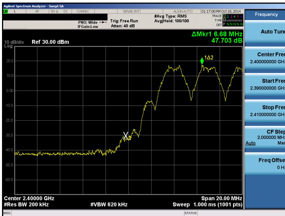
Plot 6-9. Band Edge Plot (Hopping Enabled)
