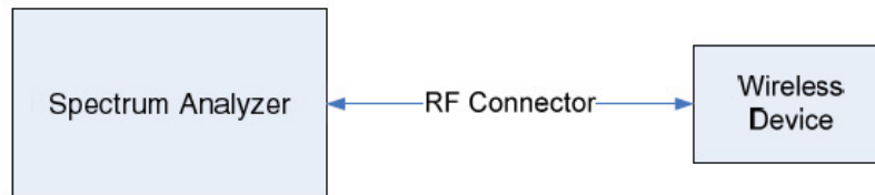
Figure 6-2. Test Instrument & Measurement Setup
