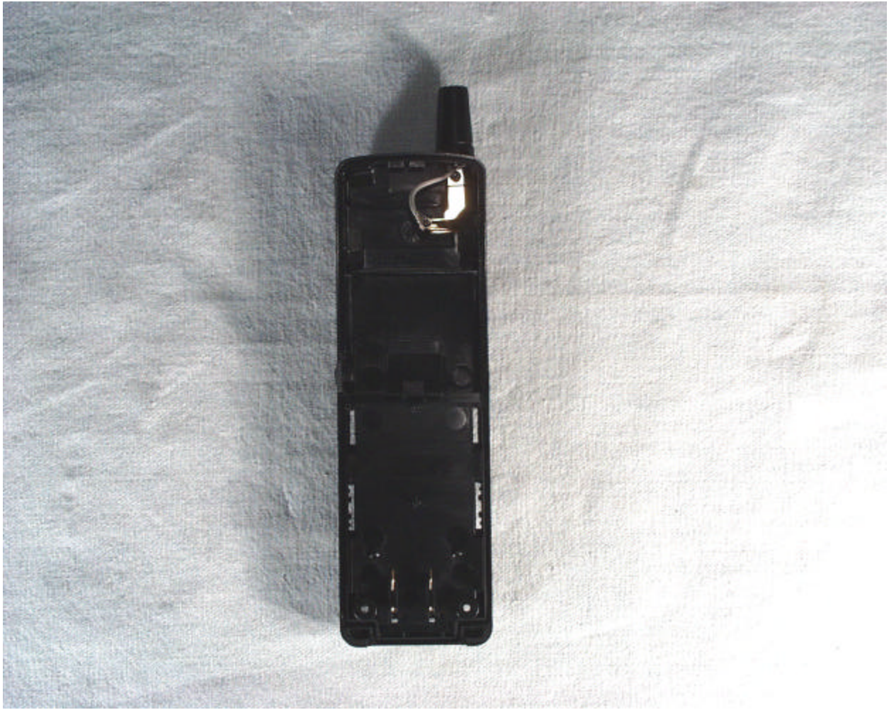
Back cover showing the antenna
