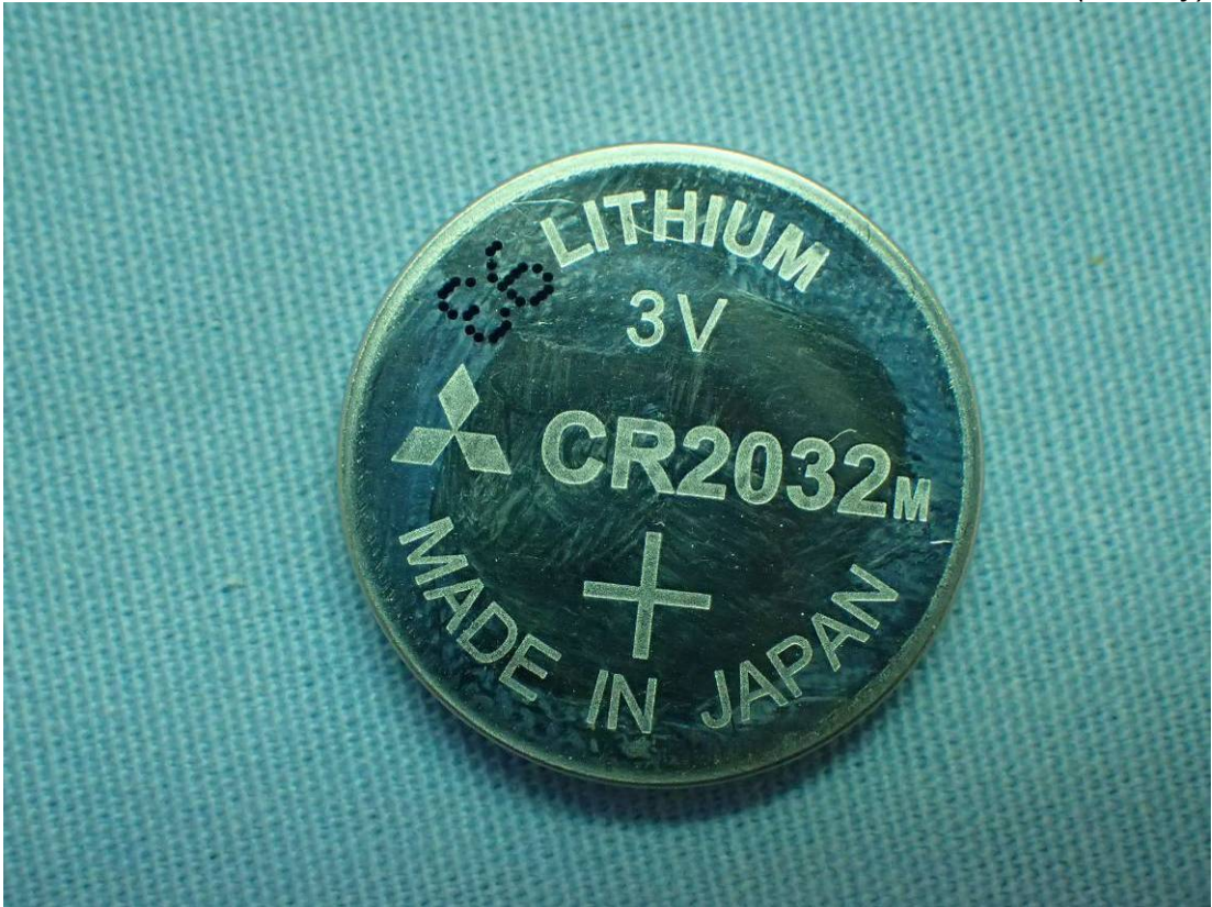
Figure 6 Internal View (Battery)
