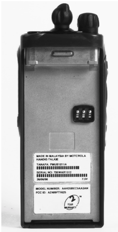
Back view of radio with battery removed showing FCC label location
