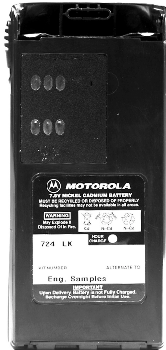
View of battery pack showing label and mating contacts to radio
