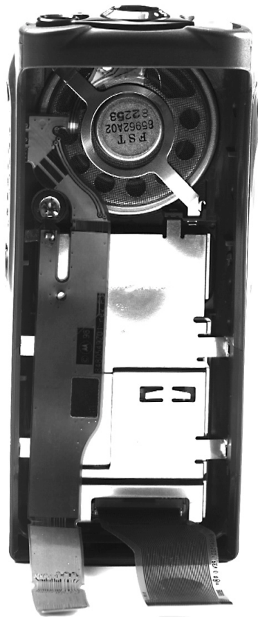
Back view of the front housing showing keypad board installed
