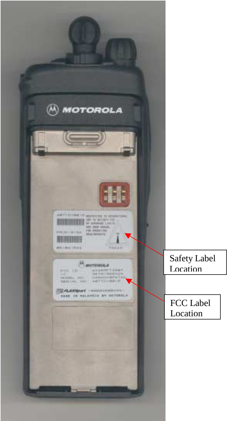
Figure 3-7: Rear view of radio showing FCC & Safety labels location
