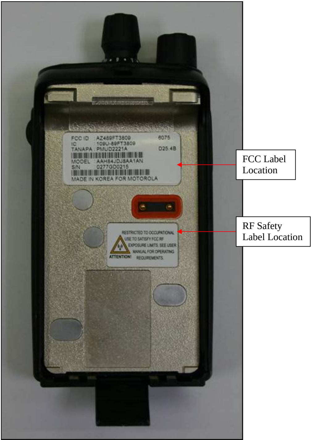
Figure 3-5: Rear view of complete radio showing FCC Label & RF Safety Label location
